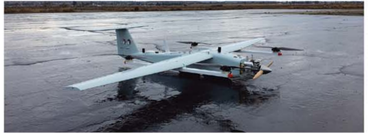
Here, the Scout Ultra is integrated with the Phoenix TerraHawk CW-20 , which combines fixed-wing speed and stability with VTOL safety and convenience.
