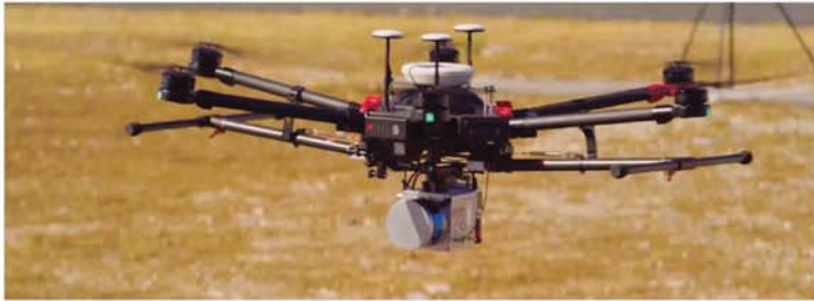
The Scout Ultra is often integrated with DJI's M600 Pro UAV, one of the most popular aircraft systems for UAV LiDAR.
